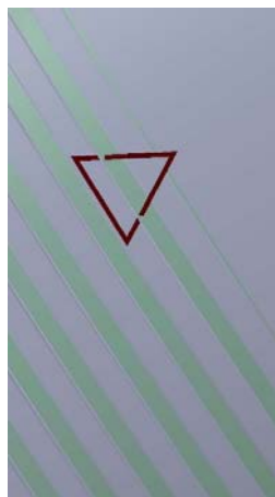
Accept: Triangle on pipe OD or Triangle tip and base on the crest.
