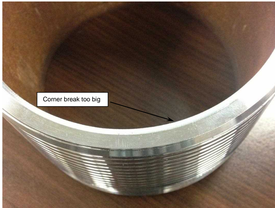
Photograph showing too aggressive ID corner break using a button tool
